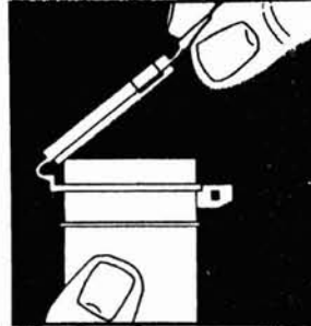
FIG. 2 Grab Lock-N-Seal Latch and move lid away from collection stream. Exercise care not to touch inside of lid or vial.
